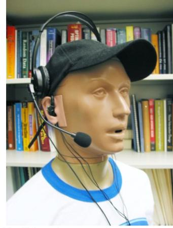
Figure 2. HATS with microphone array and headset.
