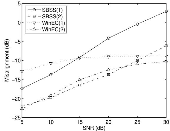
**Fig. 5.** Average misalignment when used with additive white Gaussian noise while varying SNR for one (1) or two (2) far-end talkers.
