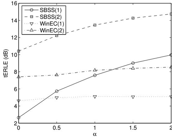
**Fig. 2.** Average tERLE when used with half-wave rectifying decorrelation nonlinearity while varying the distortion factor  $\alpha$  for one (1) or two (2) far-end talkers.
