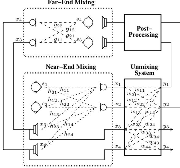
**Fig. 1.** Configuration for stereophonic teleconferencing and semi-blind source separation (SBSS).
