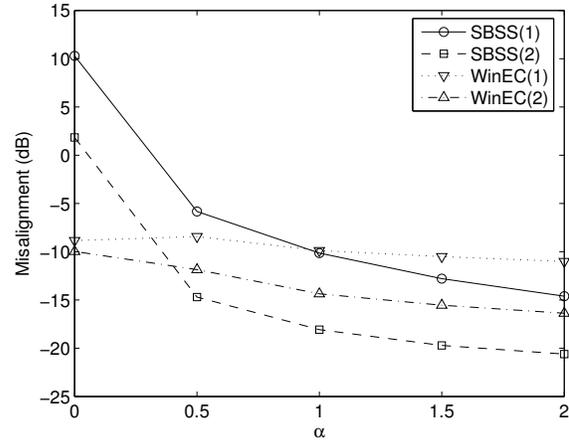
**Fig. 4.** Average misalignment when used with half-wave rectifying decorrelation nonlinearity while varying the distortion factor  $\alpha$  for one (1) or two (2) far-end talkers.
