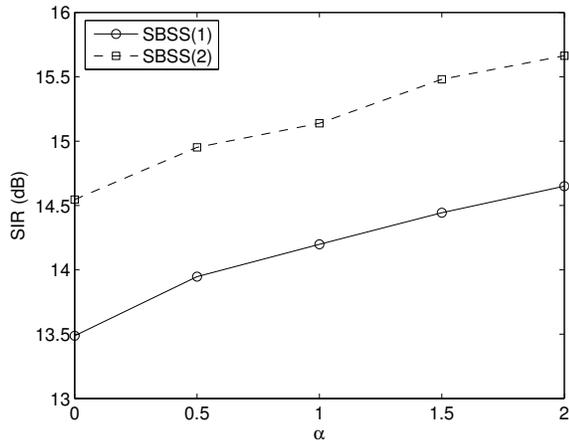
**Fig. 6.** Average SIR when used with half-wave rectifying decorrelation nonlinearity while varying the distortion factor  $\alpha$  for one (1) or two (2) far-end talkers.
