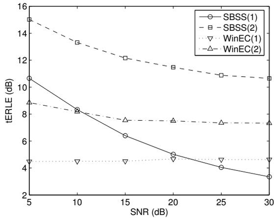
**Fig. 3.** Average tERLE when used with additive white Gaussian noise while varying SNR for one (1) or two (2) far-end talkers.
