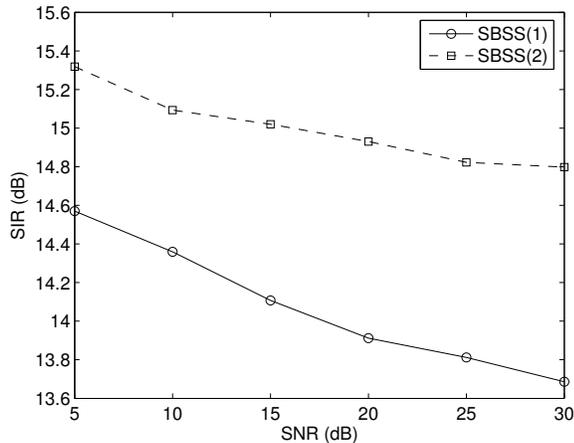
**Fig. 7.** Average SIR when used with additive white Gaussian noise while varying SNR for one (1) or two (2) far-end talkers.
