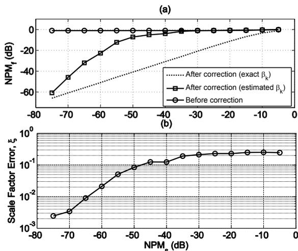
**Fig. 2.** Varying levels of subband NPM vs. (a) full-band NPM before correction, after correction with the proposed method and after correction with the ideal coefficients and (b) scale factor error.
