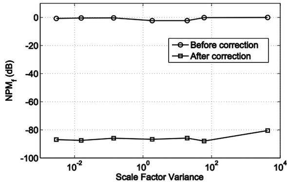
**Fig. 1.** Full-band NPM vs. scale factor variance before and after scale factor correction. The subband NPM is assumed to be  $\text{NPM}_s = -\infty$  dB.
