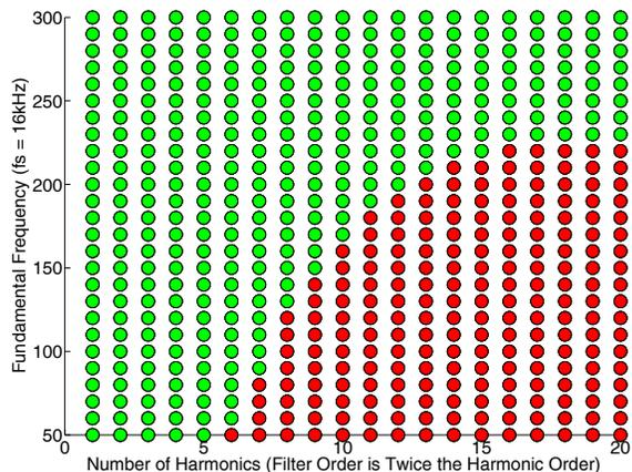
**Fig. 2.** IIR Comb Filter Stability. Green represents stable parameters and red represents unstable parameters.
