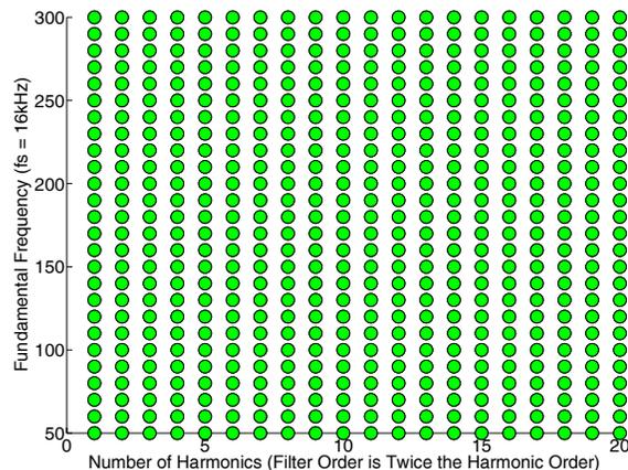
**Fig. 3.** Coherent Modulation Comb Filter Stability. Green represents stable parameters and red represents unstable parameters.
