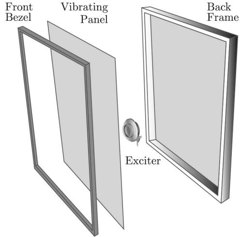
Fig. 4. Block diagram of a Distributed Mode Loudspeakers with only one exciter (wiring is omitted).
