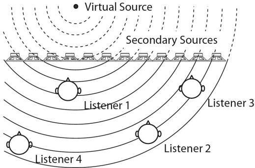
Fig. 1. Several listeners in an extended area perceive a virtual source with spatial fidelity.
