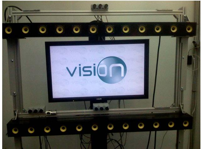
Fig. 2. Prototype combining two WFS arrays of cone loudspeakers with a 42" autostereoscopic screen.
