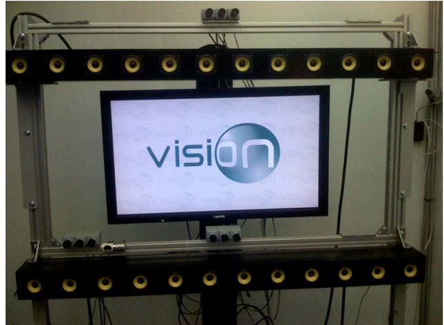
Fig. 2. Prototype combining two WFS arrays of cone loudspeaker with a 42'' autostereoscopic screen.
