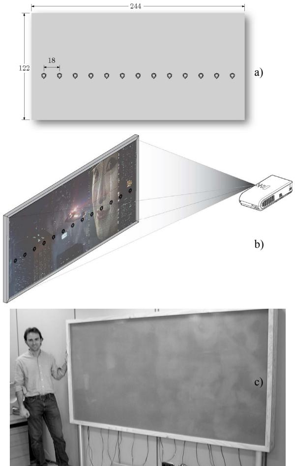
Fig. 5. Large MAP, a) block diagram and measures, b) employment in conjunction with a projector, c) photograph of the resulting prototype panel assembled and ready for use.
