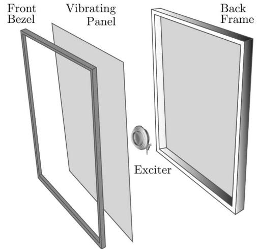
Fig. 4. Block diagram of a Distributed Mode Loudspeakers with only one exciter (wiring is omitted).
