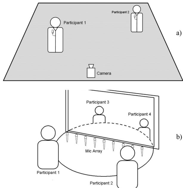
Fig. 3. Sound capture system, a) using spot-mics and the support of a videocamera and b) using a microphone array and beamforming.
