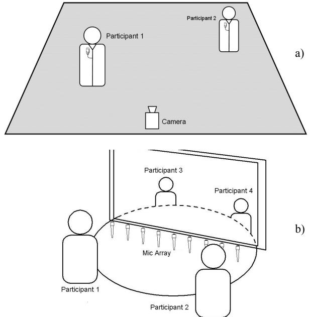
Fig. 3. Sound capture system, a) using spot-mics and the support of a videocamera and b) using a microphone array and beamforming.
