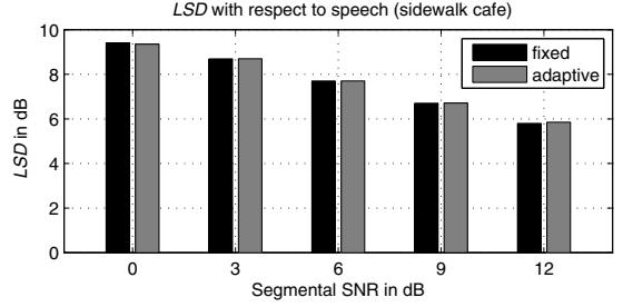
**Fig. 3.** Measured log-spectral distance (LSD) for speech.
