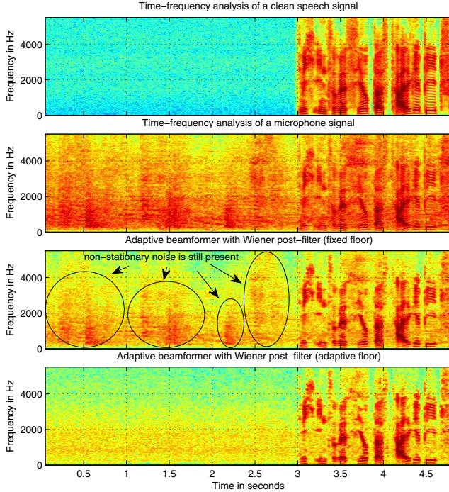
**Fig. 2.** Example of time-frequency analyses with input SNR=3 dB in an acoustical environment of a sidewalk cafe.
