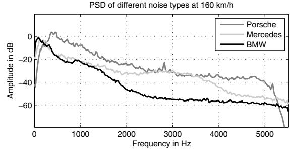
**Fig. 1.** Mean PSDs of background noises measured in different vehicles at a speed of 160 km/h.
