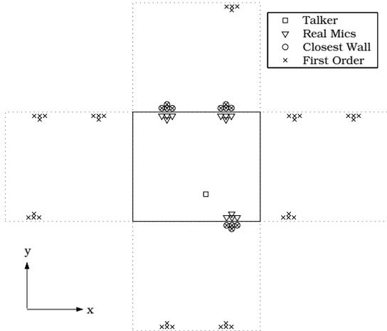
**Fig. 3.** Original microphone locations and their virtual counterparts for the real data scenario are presented here. Actual room (*solid lines*) is mirrored with each of its walls and resulting images are shown (*dotted lines*). The set of virtual microphones used by the closest wall approach is included in the set used by the complete first order reflection method.
