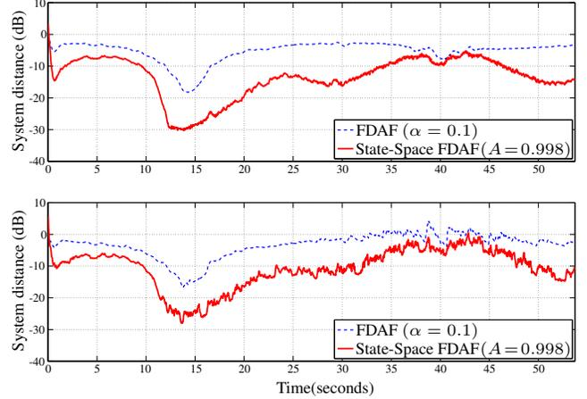
**Fig. 6.** Time-varying echo path simulation: (Upper) Single-talk; (Lower) Double-talk.
