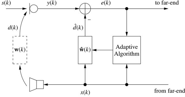
Fig. 1. Acoustic front-end, e.g., of a hands-free telephone.
