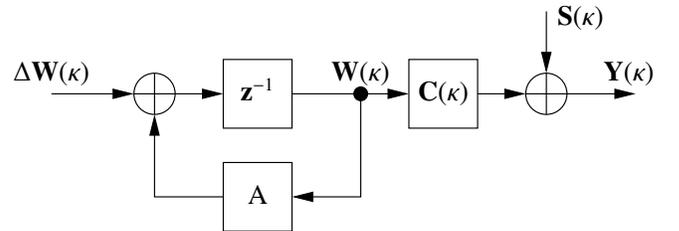
Fig. 2. Stochastic state-space model of the unknown time-varying echo path  $\mathbf{W}(\kappa)$  in the block frequency-domain.
