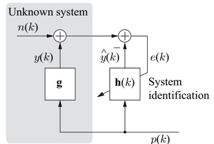
Fig. 1. Single-channel system identification with PSEQs.
