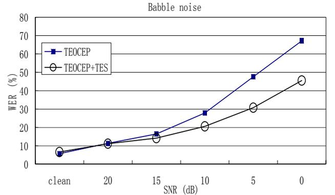
**Figure 2.** The recognition rates of Mandarin digits string recognition task with TEOCEP and TEOCEP+TES for various SNR levels in Babble noise
