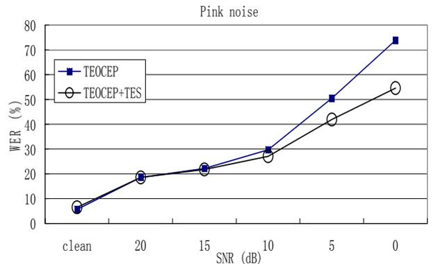
**Figure 3.** The recognition rates of Mandarin digits string recognition task with TEOCEP and TEOCEP+TES for various SNR levels in Pink noise
