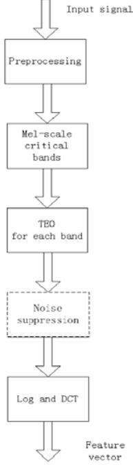
**Figure 1.** Block diagram of the TEOCEP feature
