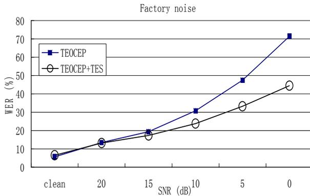
**Figure 4.** The recognition rates of Mandarin digits string recognition task with TEOCEP and TEOCEP+TES for various SNR levels in Factory noise
