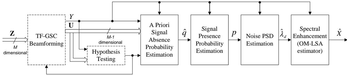
Fig. 2. Block diagram of the multichannel postfiltering.
