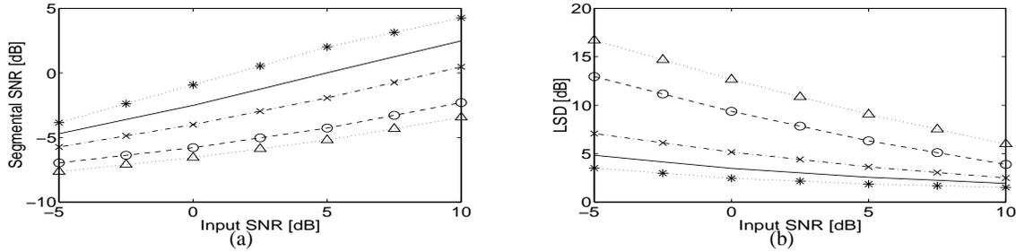
**Fig. 3.** (a) Average segmental SNR, and (b) average log-spectral distance, at ( $\Delta$ ) microphone #1, ( $\circ$ ) TF-GSC output, ( $\times$ ) single-channel postfiltering output, (solid line) multichannel postfiltering output, and ( $*$ ) theoretical limit postfiltering output.
