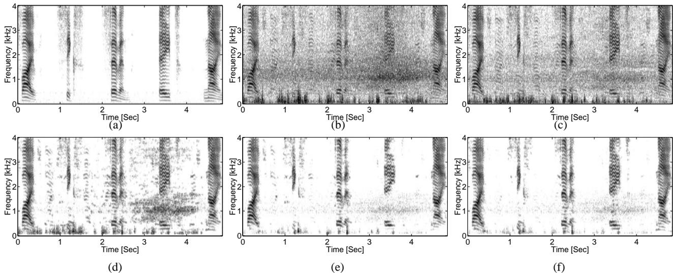
**Fig. 4.** Speech spectrograms. (a) Original clean speech signal at microphone #1: “Five six seven eight nine.”; (b) Noisy signal at microphone #1 (SNR =  $-0.9$  dB, SegSNR =  $-6.2$  dB, LSD =  $15.4$  dB); (c) TF-GSC output (SegSNR =  $-5.3$  dB, LSD =  $12.2$  dB); (d) Single-channel postfiltering output (SegSNR =  $-3.8$  dB, LSD =  $7.4$  dB); (e) Multichannel postfiltering output (SegSNR =  $-1.3$  dB, LSD =  $4.6$  dB); (f) Theoretical limit (SegSNR =  $-0.4$  dB, LSD =  $4.0$  dB).
