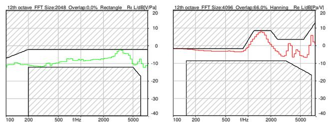
Figure 2.3: Frequency responses of selected headset and tolerance schemes; sending (left, [1]) and receiving (right, [10])
