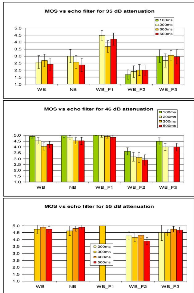
Figure 3.1: MOS results vs. echo shaping filter
