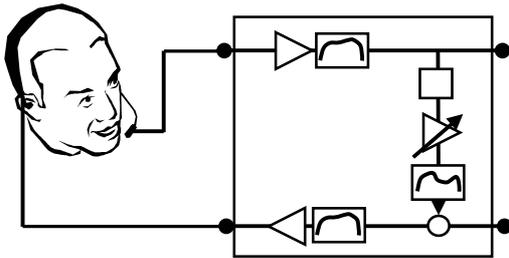
Figure 2.1: Block diagram of echo simulator
