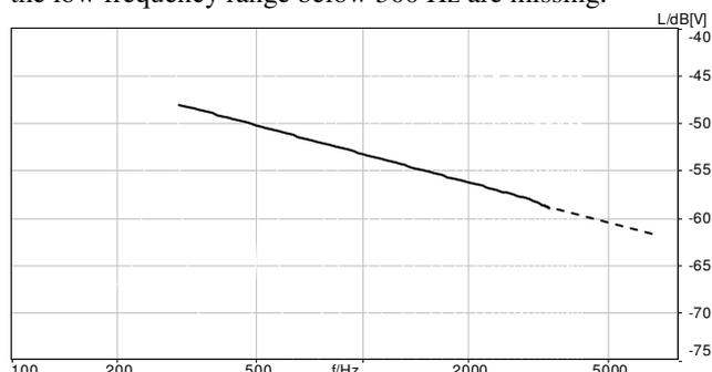
Figure 1.1:  $TCL_w$  weighting function (from [4]); dashed line: extension for wideband  $TCL_w$  calculation
