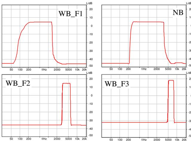
Figure 2.4: Gain functions of echo shaping filter
