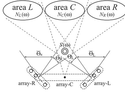
Figure 2: Area division using beamforming
