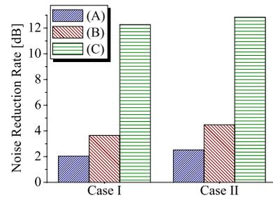
Figure 7: Noise reduction rate (A) delay-sum (B) SPB output (C) proposed method
