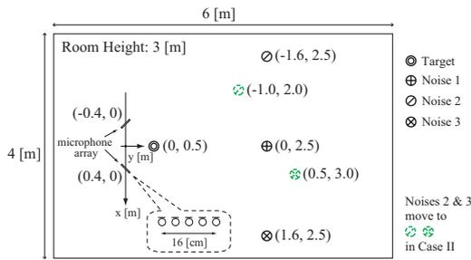
Figure 5: Sound source and microphone array arrangement
