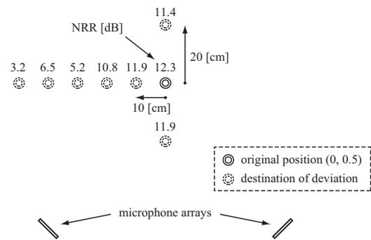
Figure 8: NRRs for the target source deviated from the original position
