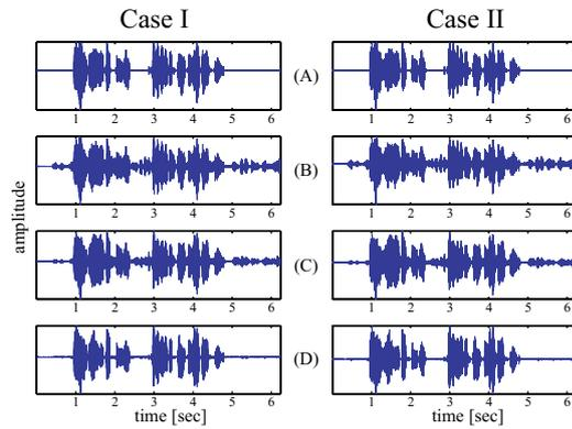
Figure 6: Sound waveforms (A) original target signal (B) measured signal (C) delay-sum beamforming (D) proposed method
