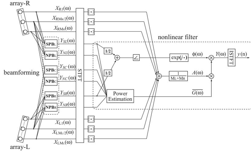
Figure 4: Signal flow of proposed method
