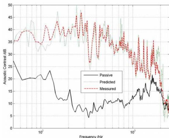
Figure 4 – Predicted and measured acoustic contrast achieved using a real-time implementation of the (adaptive) direct cancellation method in a small room
