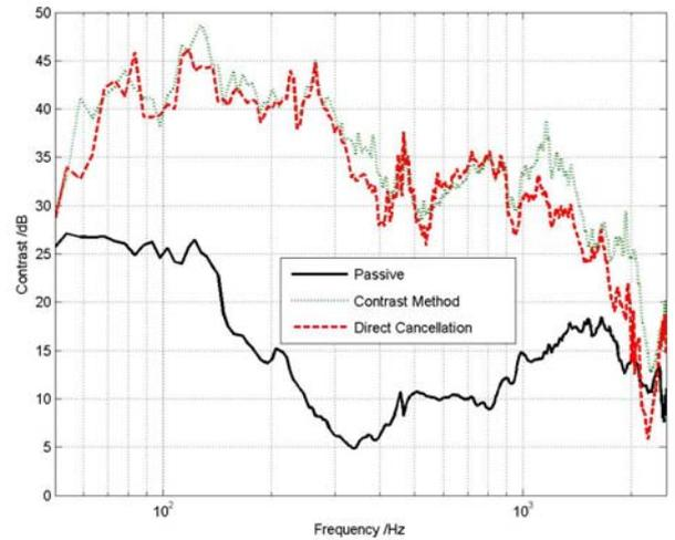
Figure 3 – Predicted acoustic contrast using the contrast method and direct cancellation from measurements obtained in an anechoic chamber
