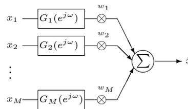
Figure 1: A general beamformer structure.
