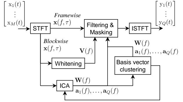
Figure 2: System structure for a real-time implementation
