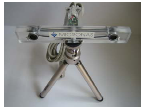
Figure 2: Two-element microphone array with Micronas UAC 3576B.
