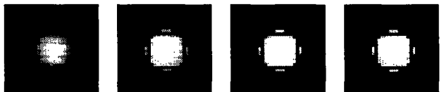
Figure 7: Applications of the extreme sharpening operator for 2, 4 and 8 iterations using a parabolic structuring function q^\rho(x) with \rho = 1.0 .
