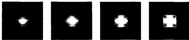
Figure 8: Applications of the extreme sharpening operator for 2, 4 and 8 iterations using a 4-connected flat structuring function with \rho = 1.0 .
