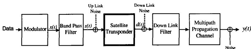
Fig. 1 : mobile satellite channel
