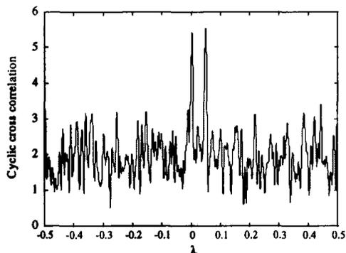
Fig. 2. Initial Estimation of the Doppler frequencies.  $N = 128$
