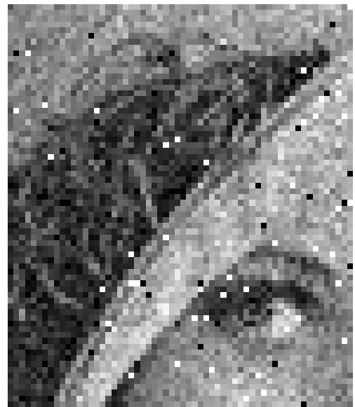
Fig.4 (a) Noisy image (Gaussian \sigma = 20 , Impulse 2%)
