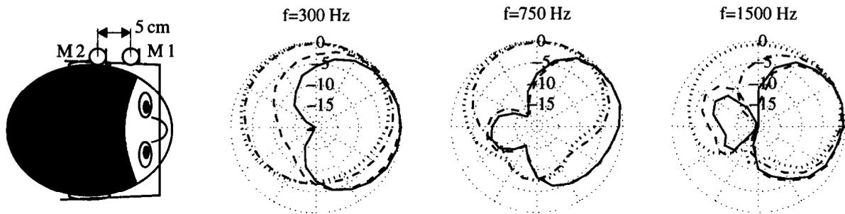
Figure 4: Arrangement of the microphones beneath the dummy head and the measured directivity pattern in dB:
