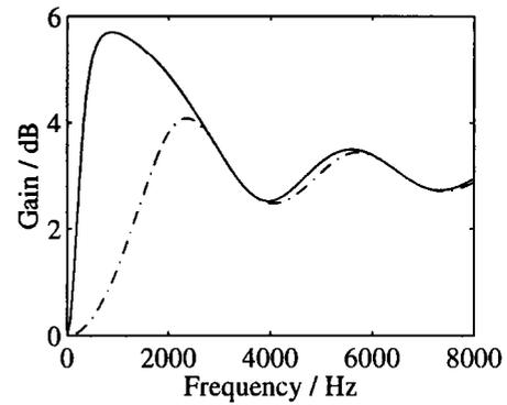
Figure 2: Gain (according to equation (2)) of end-fire arrays with two omnidirectional microphones, placed at a distance of 5 cm
