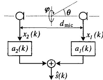
Figure 1: Structure of an array with two microphones
